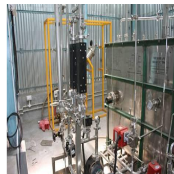
1000 LPD ceramic membrane based reactor for grey water
