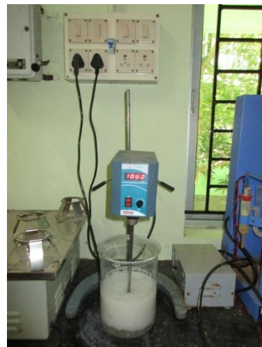
Fig. 3 Recycled plastic waste treated with sodium hydroxide using mechanical stirrer
